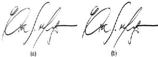
Figure 1. Histogram equalization: (a) Signature captured without equalization, (b) Signature captured with equalization.
